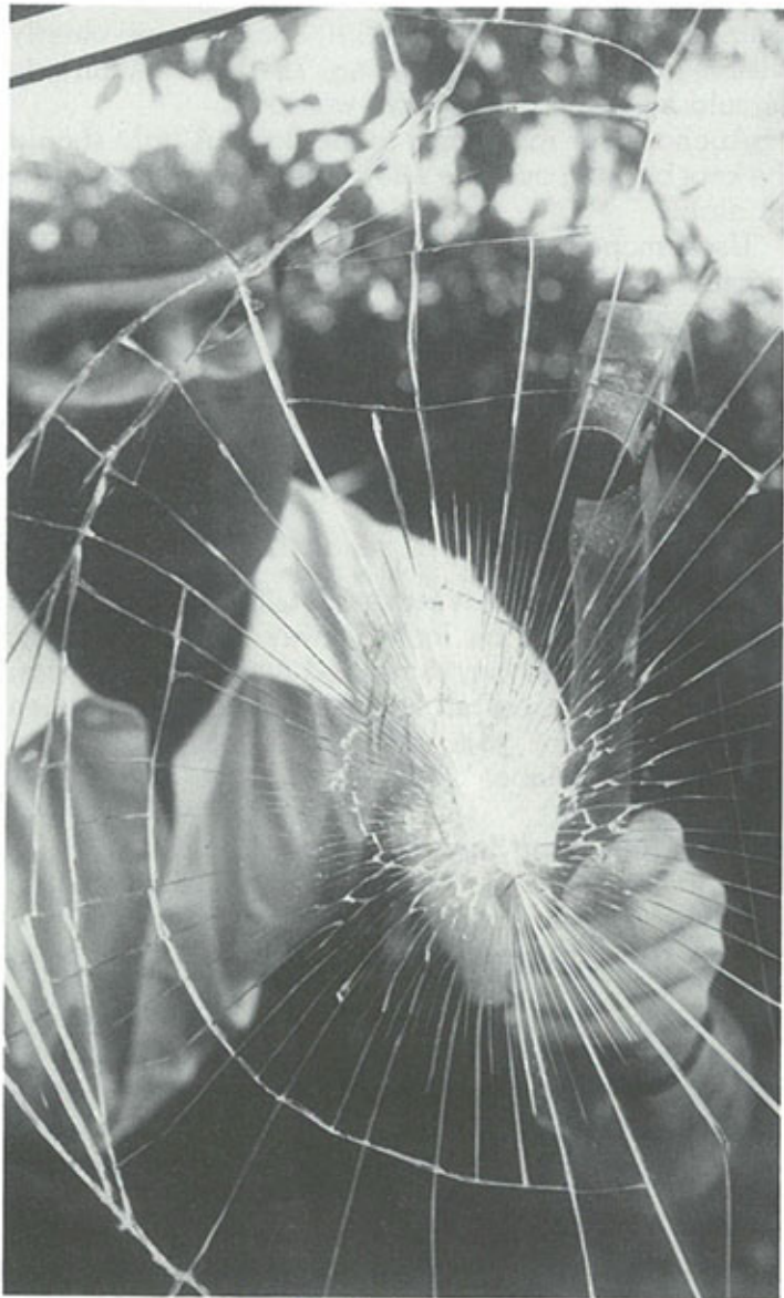
Shatter-resistant security film is a good deterrent against vandalism and "smash and grab" offences.
